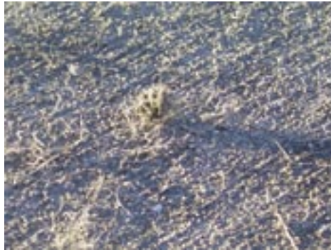
Unsightly balling and fuzz from fibrillated polypropylene
