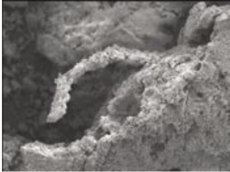
UltraFiber 500 readily bonds to cement
