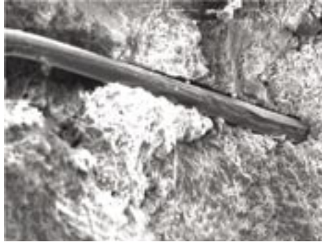
Synthetic fibers exhibit minimal bonding to cement
